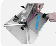
Cartridge wedges Quick loading and change of wedge size
